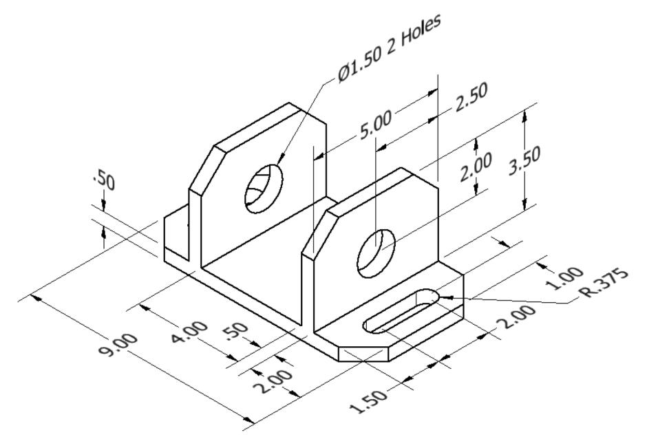
Notes: Chamfers are 1" by 1" Typical Slots on both sides
